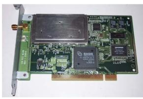
The 2.4GHz radio and modem is integrated into a US\$150 wireless LAN card. It is fairly similar to normal Ethernet card. The major difference is in the antenna connector pop up at the end of the card to be used to connect the coax cable and external antenna to the card. The Linux O/S driver of the card is available in public domain, such as http://www.sourceforge.org which will really help those who like to build their own infrastructure.
