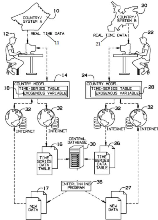
**Figure 2:** Inter-Linkage Mechanism for Distributed Simulation Models with Human Intervention
