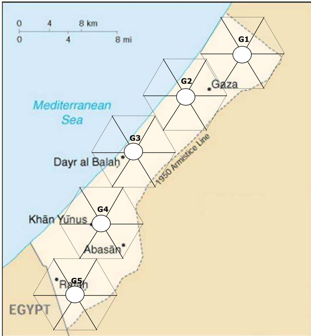
Figure 9: WiMAX network design for Gaza Strip
