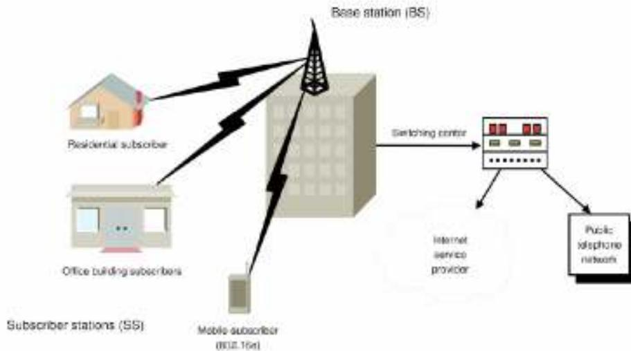
**Figure 3: A typical WiMAX Scenario to be used in the GUS/Palestine/Gaza Strip and West Bank project.**
