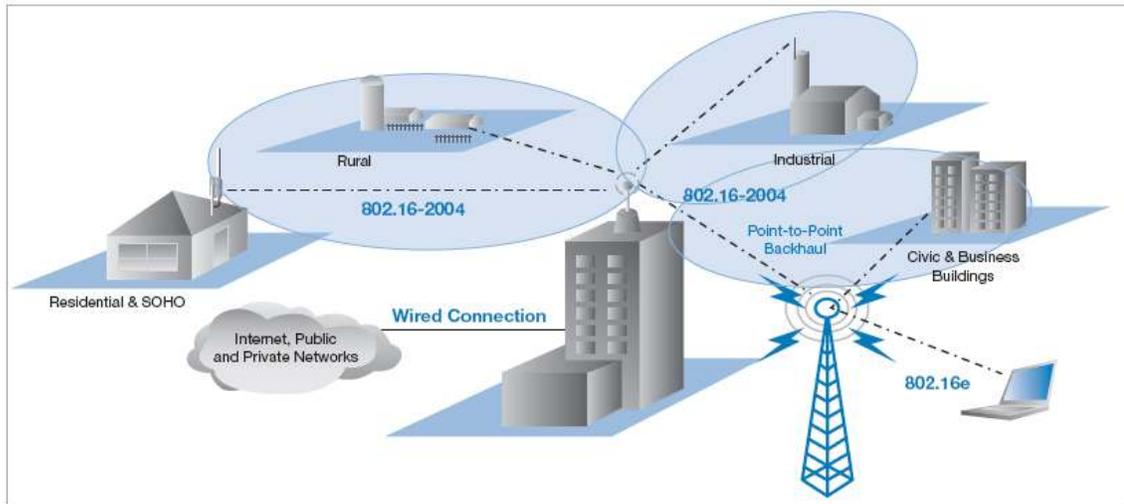
**Figure 2: Fixed WiMAX deployment and usage models.**
