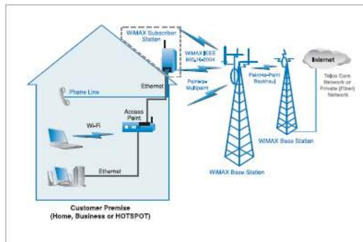
**Figure 1: WiMAX Network Topology for Fixed Access Usage Model**
