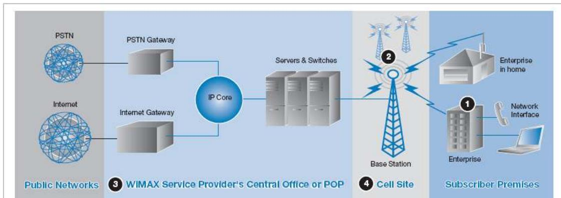
**Figure 4: a properly deployed license-exempt WiMAX solution**
