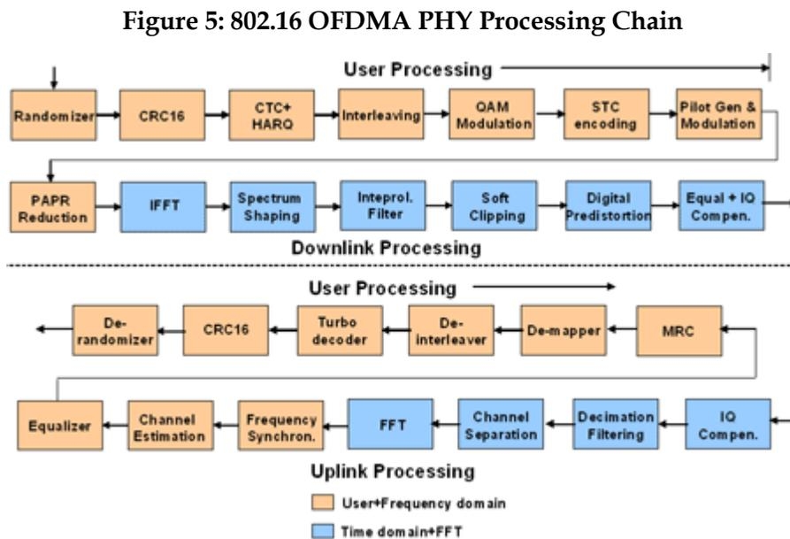
In the **downlink** process, packets arriving from the MAC layer are subject in sequence to randomization, forward error correction, and coding (such as CTC, a convolutional line coding). Then follows interleaving and modulation, and eventually a key block of any of the processing – the Inverse Fast Fourier Transform (IFFT), which moves the signal from the frequency domain to the time
